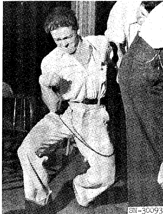
Fig. 9. Determination of the maximum current a subject can tolerate and still let go of the energized conductor.
